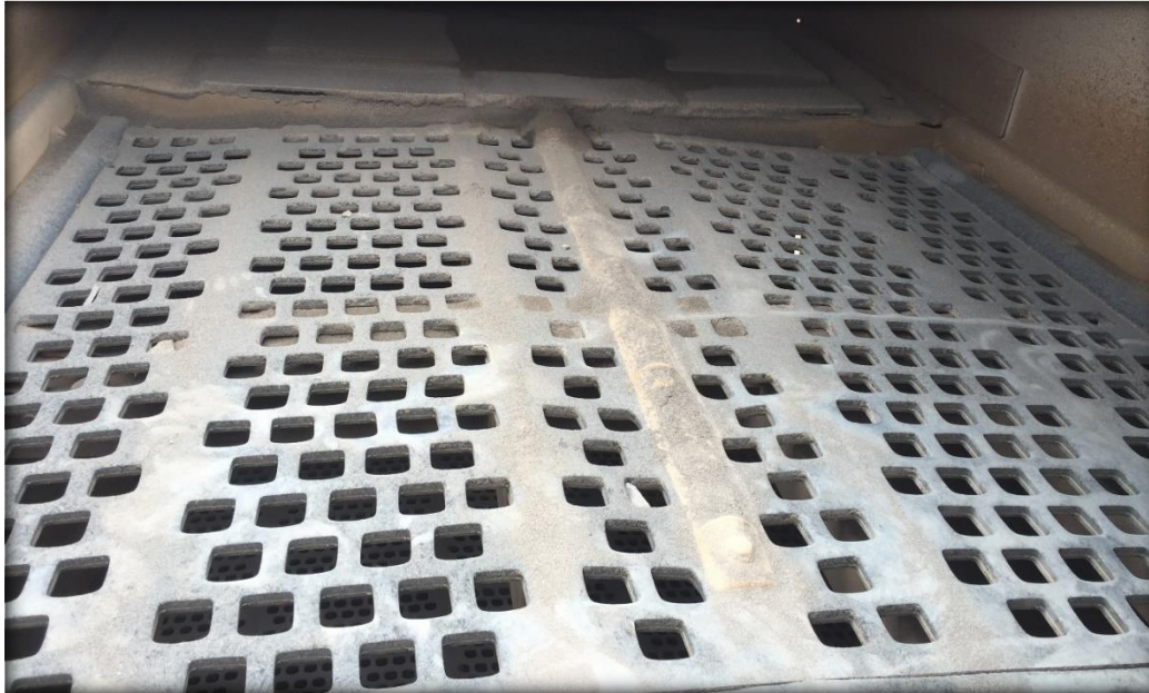
Conventional cross tensioned rubber screen cloth pre conversion
