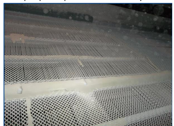
Example opened apertures with all wire style screen
