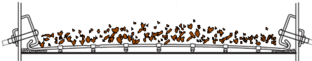
For proper screen cloth tension there must be sufficient & even crown across the whole deck
