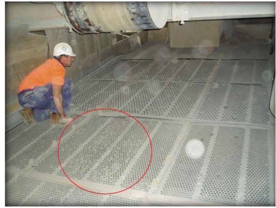
Middle section of these rubber screens are pegged, outer sections are clear. It can be very difficult to get good tension on triple camber decks
