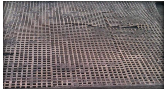
Loose poly cloth flogged-out over support bar
